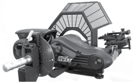
FIG:1 Lathe in upright position. Note that adjustments to cutting head are simpler in this position.
