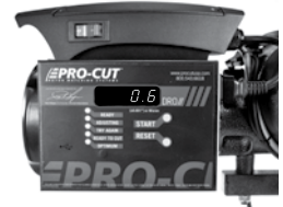
DRO computer compensated for lateral run-out to 0.0006" and ready to cut.
