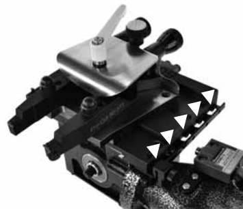
| Detail of the gib adjustment screws
