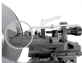
The chip deflector rides over the cutting arms as shown above. The chip deflector should be used every time.
