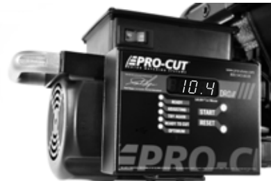
| This value represents hours and tenths of an hour that the motor has to run.
