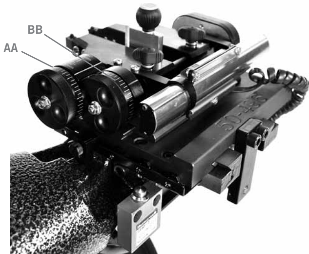
Detail of outboard adjustment knob (AA) and inboard adjustment knob (BB)
