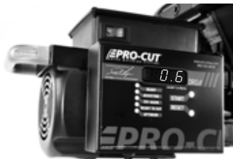
| This display of final compensation equals .0006"
