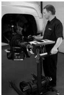
STEP 4. Technician sets cut depth. *SPINDLE GUARD 50-1740 NOT SHOWN!
