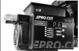
DRO computer compensated for lateral run-out to 0.0006" and ready to cut.
