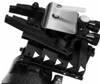
| Detail of the gib adjustment screws
