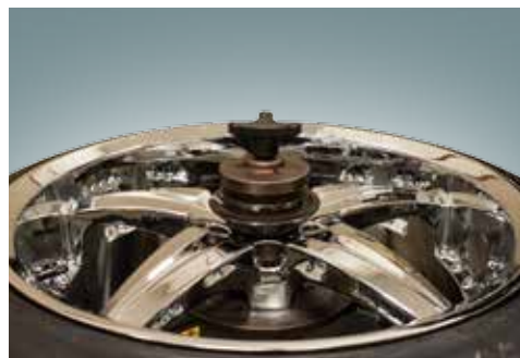
Center-post Hydraulic Clamping
