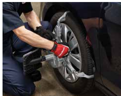
AC400 wheel clamps securely attach to tires without touching the rim; clutch-limited clamping force ensures secure and consistent attachment.
