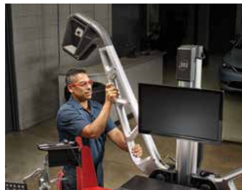
Folding camera beams provide a lower center of gravity for improved stability while protecting cameras during transport.
